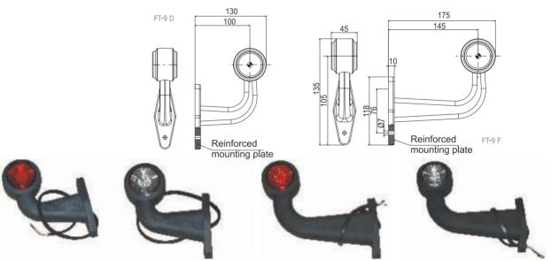
LED 2 function end outline marking lamp white/red with flexible bracket and integrated flat cable  $2x0.75 \text{ mm}^2$ . Voltage range 12-30 V DC - non-polarised. The product is fullfilling highest quality standards. Extreme small power consumption using a 12 V cirquit 12V(0.04A)=0.5W and 24 V cirquit 24V(0.04A)=1W. Working temperature range from  $-40^{\circ}\text{C}$  to  $+100^{\circ}\text{C}$ .
