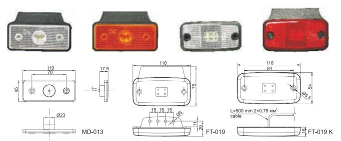
Universal amber LED side marking lamp with reflector, holding bracket and integrated cable  $2x0,75~\text{mm}^2$ . Voltage range 12-30 V DC - non-polarised. The product is fullfilling highest quality standards. Extreme small power consumption using a 12 V cirquit 12V(0,04A)=0,5W and 24 V cirquit 24V(0,04A)=1W. Working temperature range from  $-40^{\circ}\text{C}$  to  $+100^{\circ}\text{C}$ .
